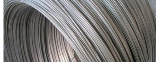
Tyre wire is extracted from the beads of the tyre Image Credit: Renecal
