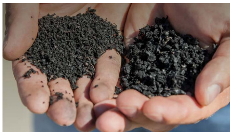
Rubber powder can be ground into various granulated sizes for different uses Image Credit: Biocaucho
