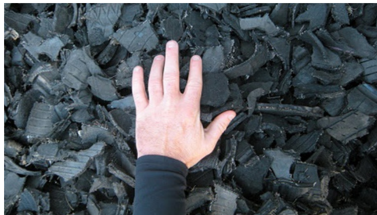
Rubber crumbs can be used as an alternative fuel source Image Credit: Flexdeal Export
