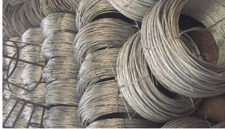
Scrap wire extracted from tyres can be re-sold for other uses Image Credit: L.B. Industries
